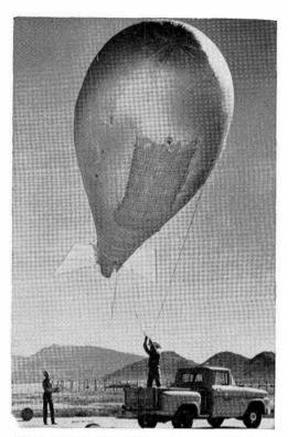
TWO BALLOONS-40 feet long and 17 feet in diameter-were tethered at 1500-foot altitude to suspend strings of pressure gages over the blast site of a recent Coyote Plowshare explosive experiment.
